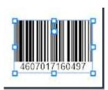
19. The default barcode type is *Auto*, which means that the type of barcode will be determined automatically (EAN 13, EAN 8, UPC A, UPC E, CODE 39 or CODE 128), depending on the length of the data and the content of certain characters in them.
